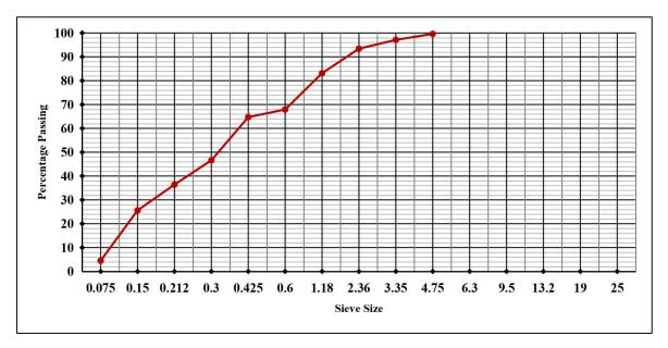
Figure 3: Result of Sieve Analysis
